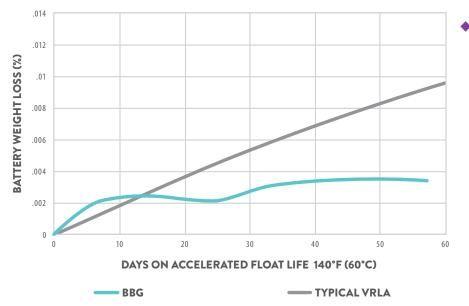
The use of permeability plastics and a balanced cell in our BBG batteries significantly help reduce water loss, which contribute to long life at high temperatures and prevent dryout.
