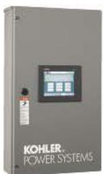
Responsible for generator and load management, the master control panel handles load add/load shed; number of gensets online; and also monitors electrical and mechanical loads along with event logging and alarms.
